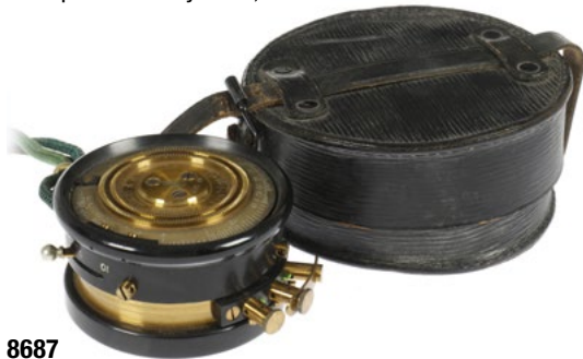
8687 Telefonbrücke nach Nippoldt, Messbereich 0.1-100 Ohm, von Hartmann & Braun, in originaler Schatulle, H 11 Nippoldts' telephone bridge, range from 0.1 to 100 ohms, made by Hartmann & Braun in original box, H 11 150,- €
